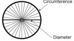
So if Andrew has a wheel with diameter 50 centimetres, its circumference would be about 150cm or 1.5 metres and it would take 100 turns of the wheel to travel a distance of 150m and 1000 turns to travel 1.5 kilometres.
